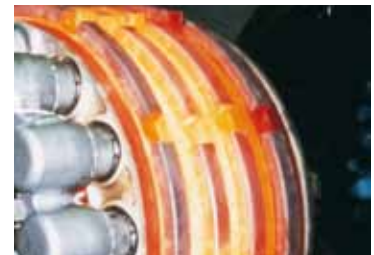
PANOX® based carbon/carbon aircraft brake disk being tested
