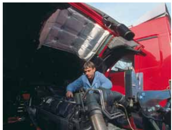
Insulation material of truck engines using nonwovens made of PANOX®
