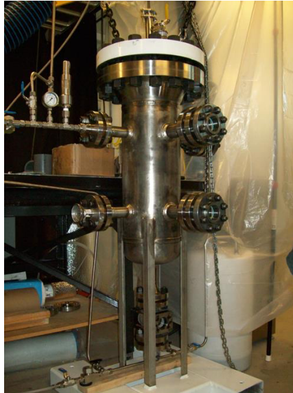
Vartega's Lab Scale Solvolysis System
